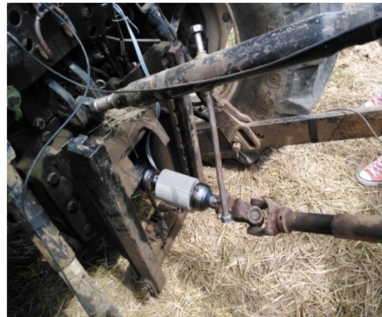
Fig. 3. Tractor torque transducer, HBM 1000 GARV beam coupled to the central tie rod
