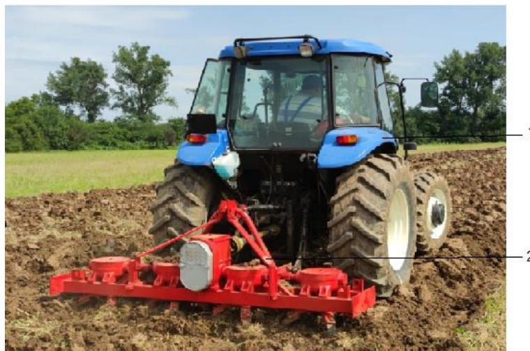
Fig. 1. Agricultural harrow unit with vertical rotor in operation:
